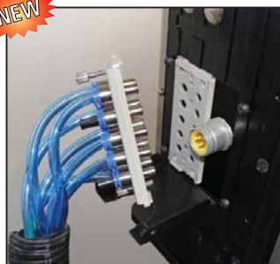
EL-NCS-AVC-EV-12 TORCH WIZARD™ for external valve bank controlled by existing air manifold on controller (cover removed)
